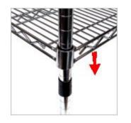
The **Plastic Shelf Clips** snap into the grooves of the Upright Post and allow the shelves to be adjusted on 25mm increments. The Shelves slide down the Upright Posts and over the Plastic Shelf Clips to lock the shelves into position.
